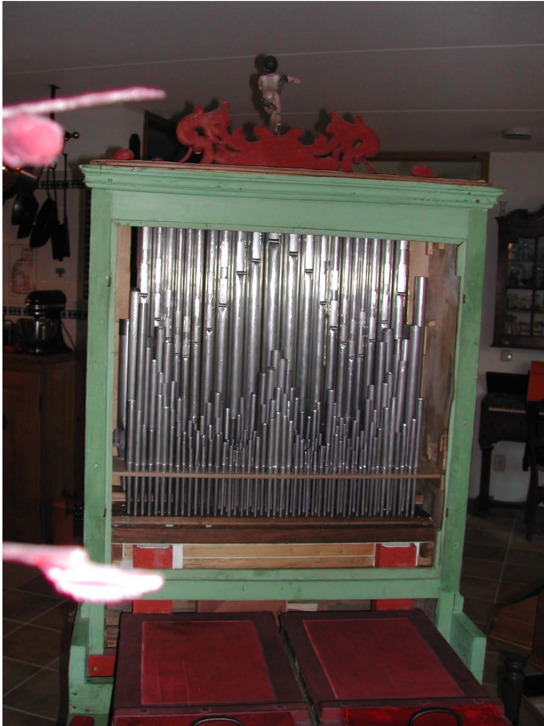
New ranks of pipes: from backside (closest to the camera) 1 ft; quint 1 \frac{2}{3} ; octave 2 ft; prestant.
