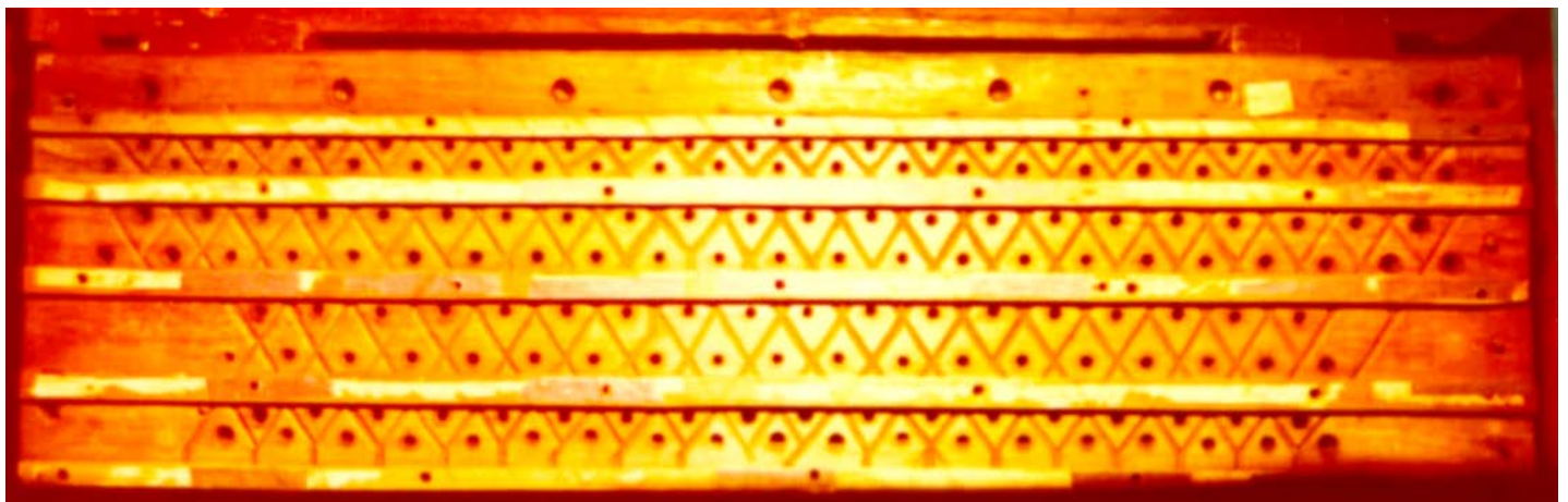
sliders removed, pictures also showing holes for bass octave 4ft
