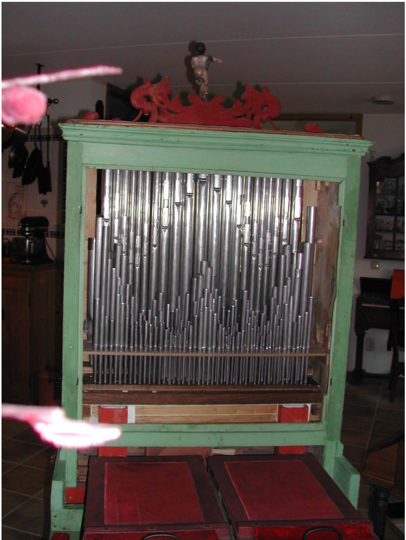
new ranks of pipes: from backside (closest to the camera) 1'; fifth 1½'; 2'; principal 4'
